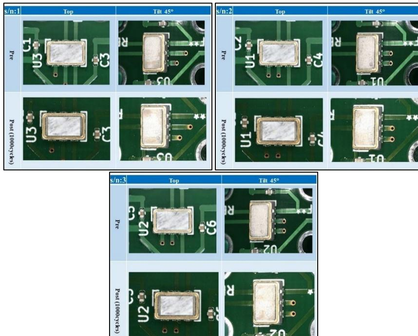
Fig. 30. The results of the external visual examination after the thermal shock test on voltage-controlled crystal oscillator
