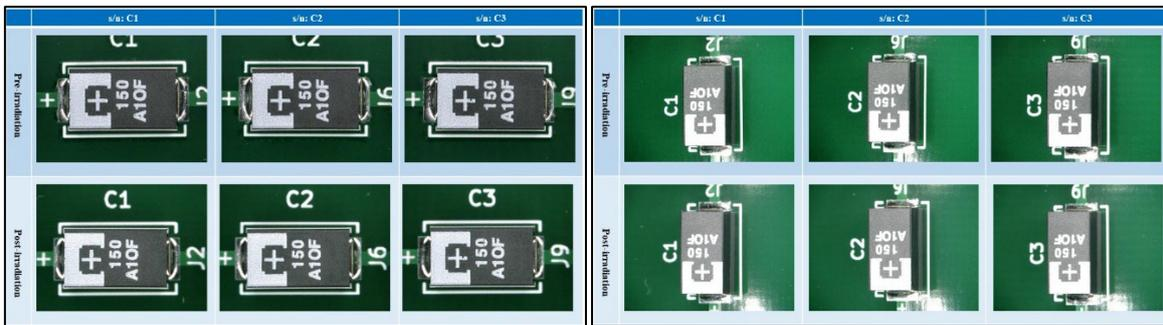
Fig. 3. the results of the external visual examination after irradiation on the polymer tantalum capacitor
