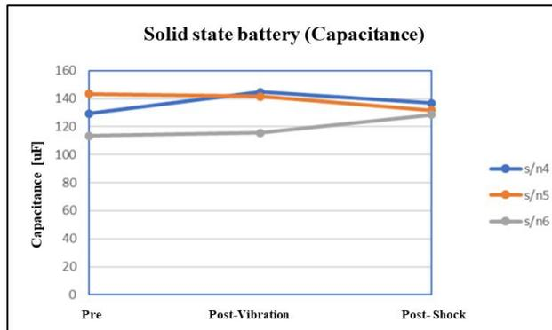
Fig. 16. The results of the mechanical stress tests on the solid-state battery
