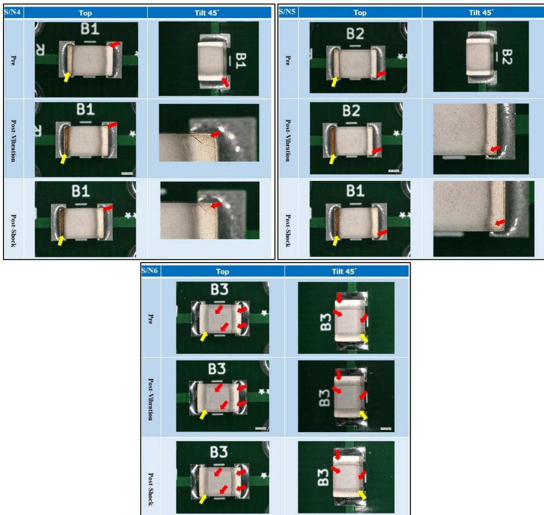
Fig. 17. The results of the external visual examination after the vibration test and the shock test on solid-state battery
