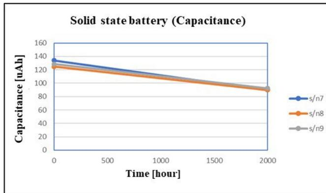
Fig. 37. The result of the electrical characteristic measurements after the ion migration test on solid-state battery
