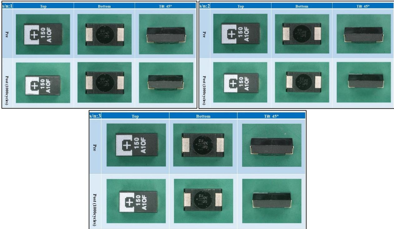
Fig. 20. The results of the external visual examination after the thermal shock test on the polymer tantalum capacitor
