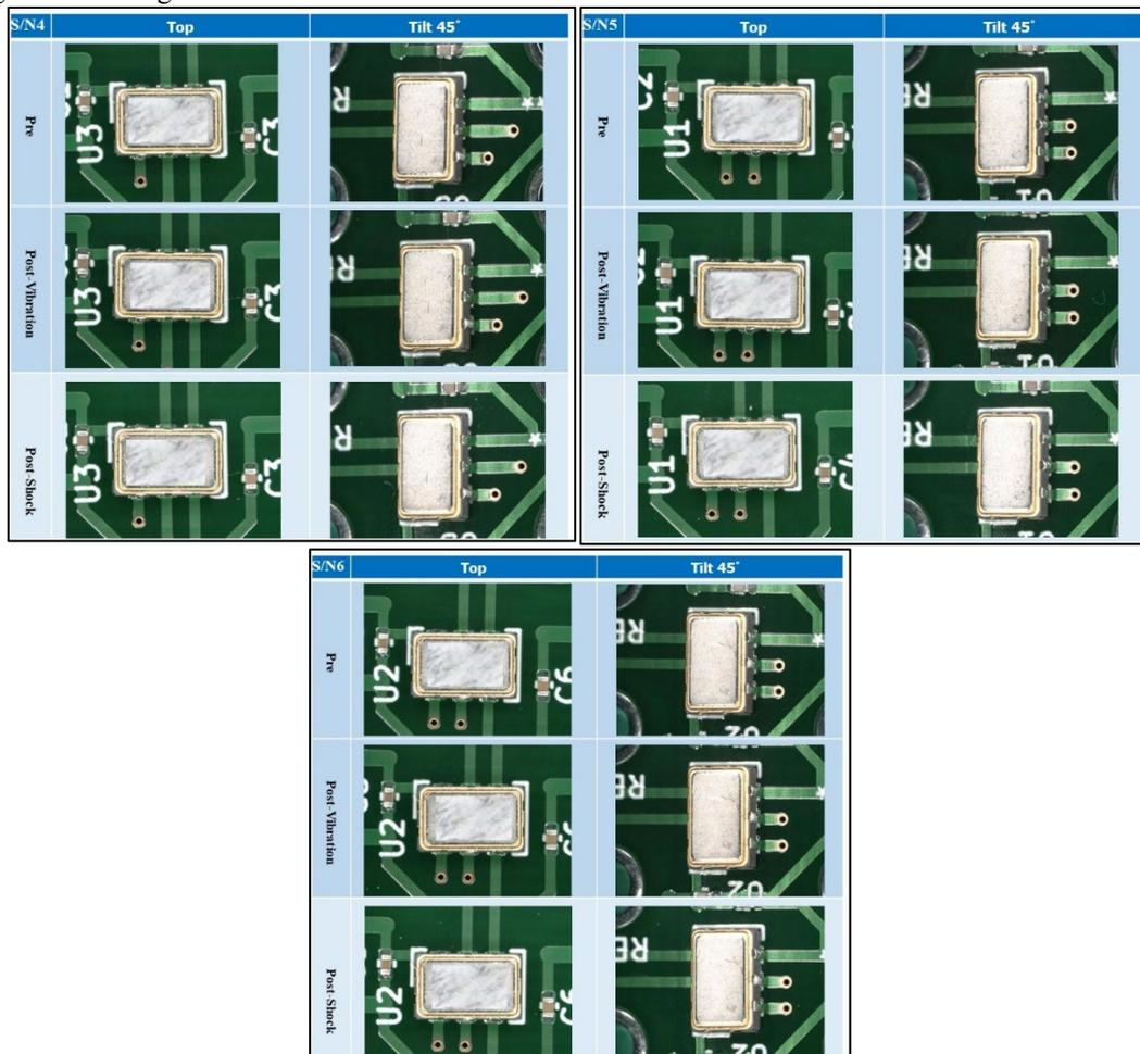
Fig. 15. The results of the external visual examination after the vibration test and the shock test on the voltage-controlled crystal oscillator
