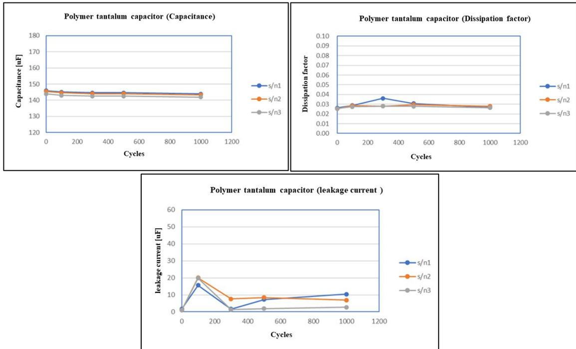
Fig. 19. The results of the electrical characteristic measurements after the thermal shock test on the polymer tantalum capacitor
