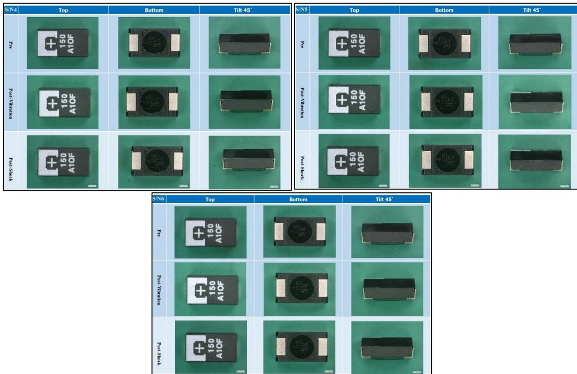
Fig. 11. The results of the external visual examination after the vibration test and the shock test on polymer tantalum capacitor
