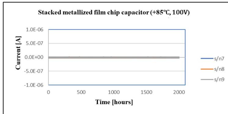
Fig. 26. The result of the ion migration test on stacked metallized film chip capacitor
