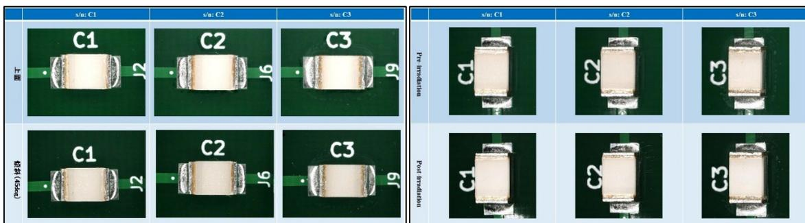
Fig. 5. The result of external visual examination after the TID test on the stacked metallized film chip capacitor
