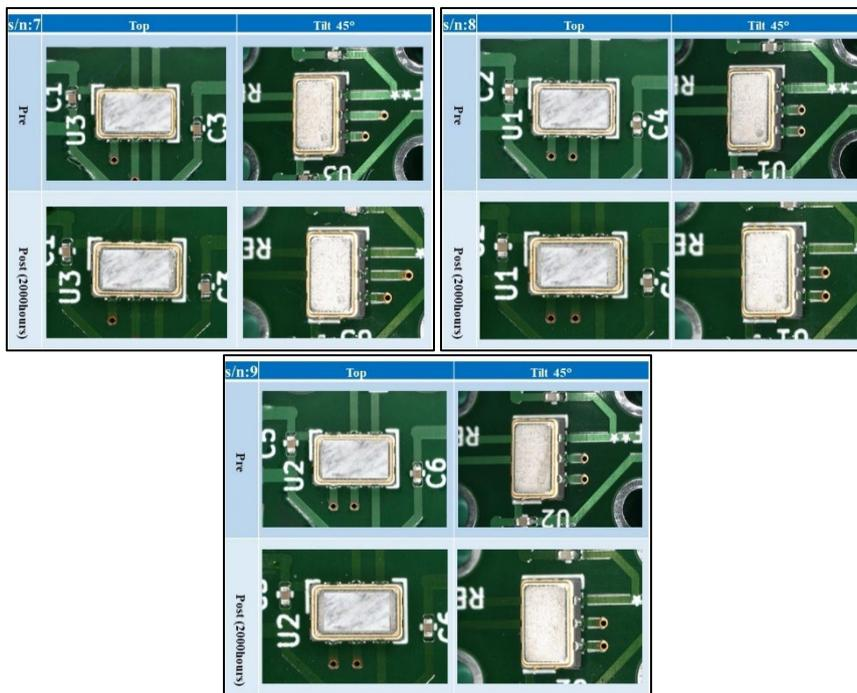
Fig. 33. The result of external visual examination after the ion migration test on voltage-controlled crystal oscillator
