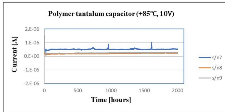
Fig. 21. The result of the ion migration test on the polymer tantalum capacitor
