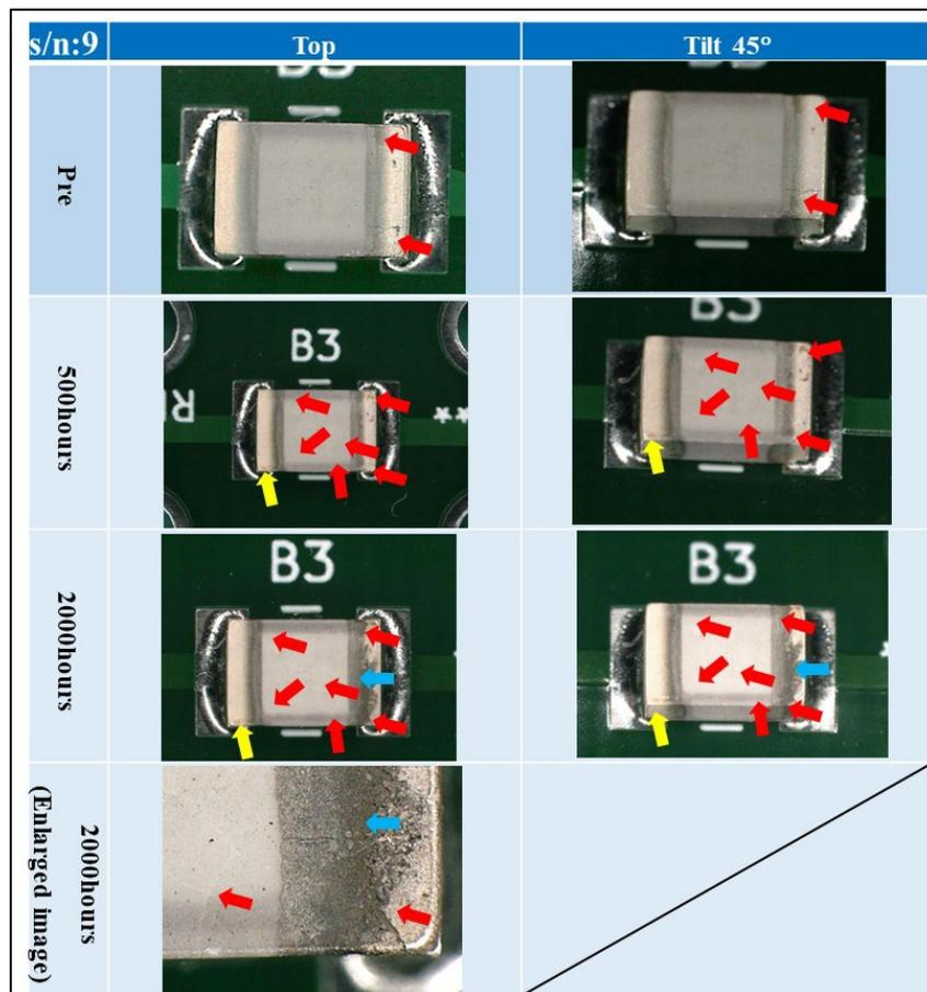
Fig. 38. The result of external visual examination after the ion migration test on solid-state battery
