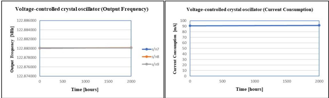
Fig. 32. The result of the electrical characteristic measurements after the ion migration test on voltage-controlled crystal oscillator
