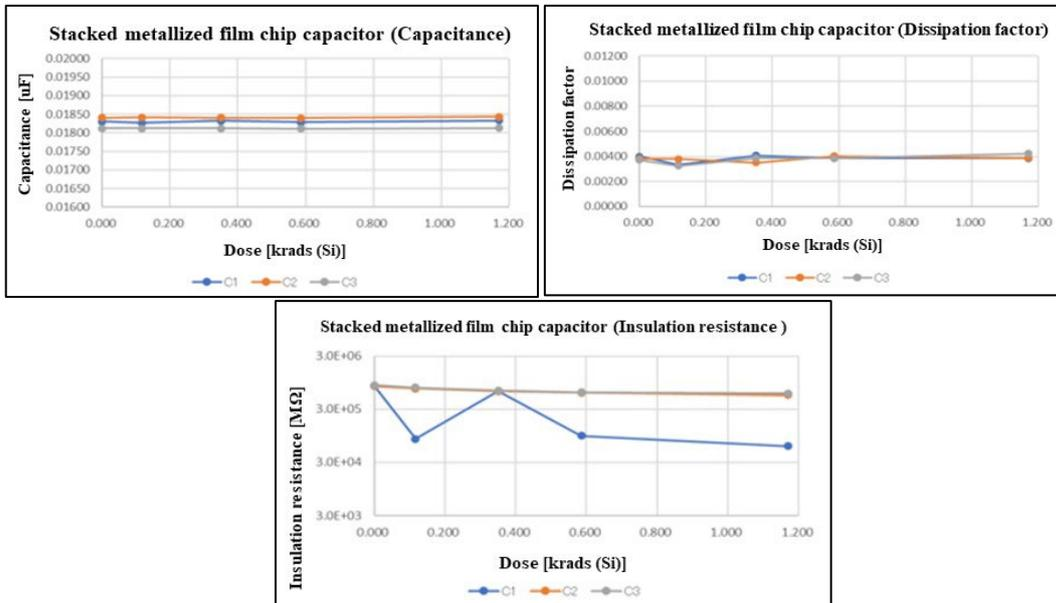
Fig. 4. The results of the electrical characteristic measurements after the TID test on the stacked metallized film chip capacitor
