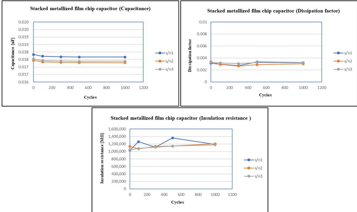
Fig. 24. The results of the electrical characteristic measurements after the thermal shock test on the stacked metallized film chip capacitor
