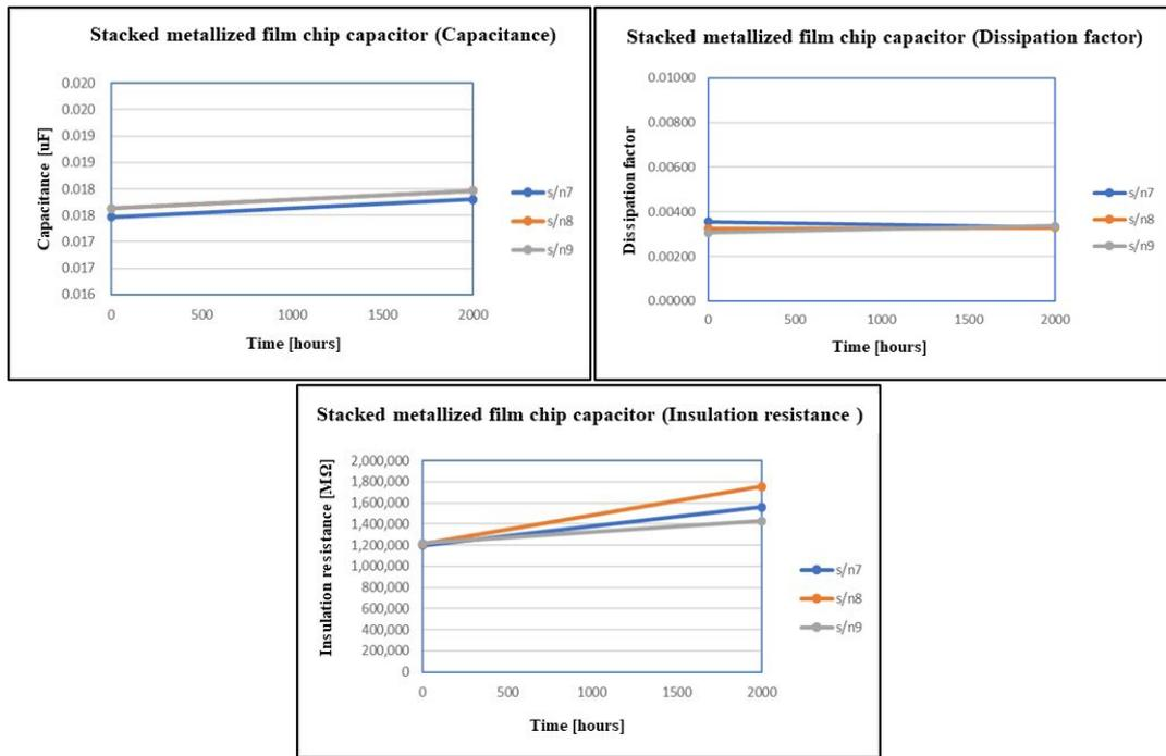
Fig. 27. The results of the electrical characteristic measurements after the ion migration test on stacked metallized film chip capacitor
