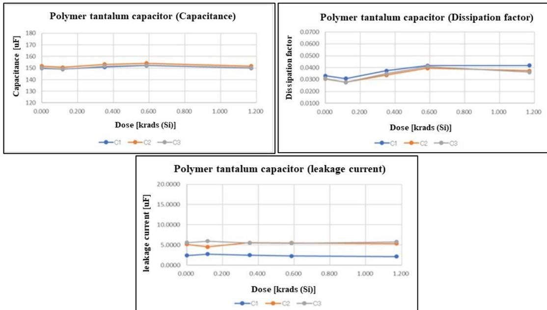
Fig. 2. The results of the electrical characteristic measurements after the TID test on the polymer tantalum capacitor
