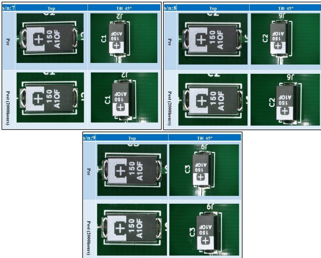
Fig. 23. The results of the external visual examination after the ion migration test on the polymer tantalum capacitor
