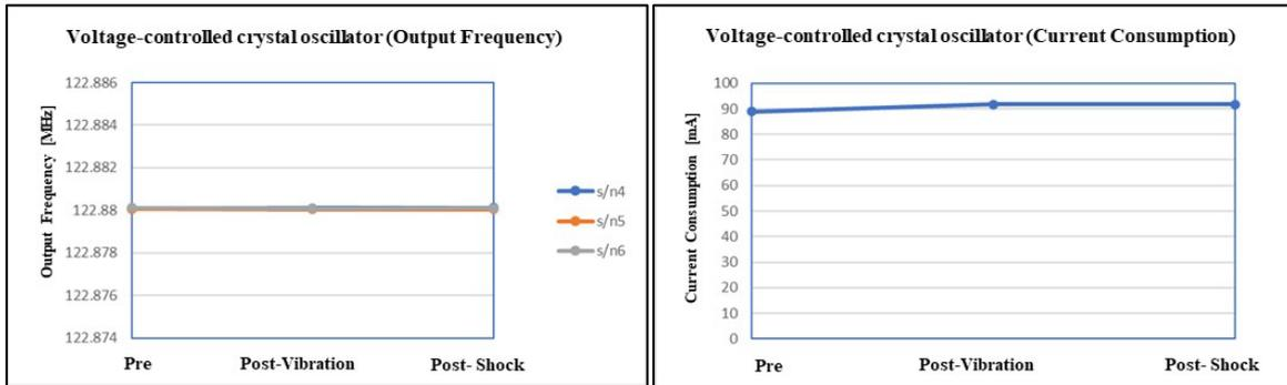
Fig. 14. The results of the electrical characteristic measurements after the vibration test and Shock test on the voltage-controlled crystal oscillator
