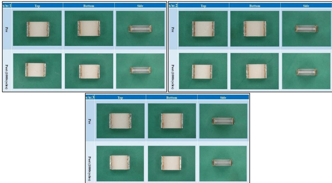
Fig. 25. The results of the external visual examination after the thermal shock test
