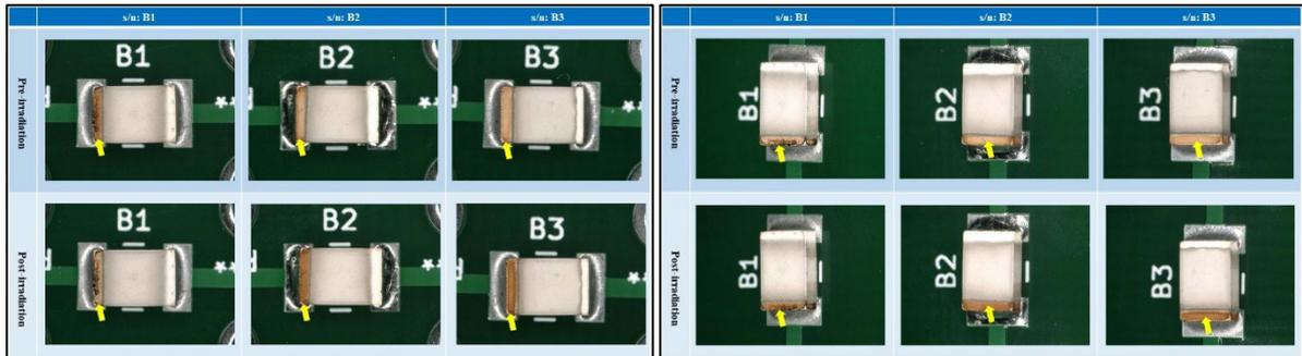
Fig. 9. The result of external visual examination after the TID test on solid-state battery
