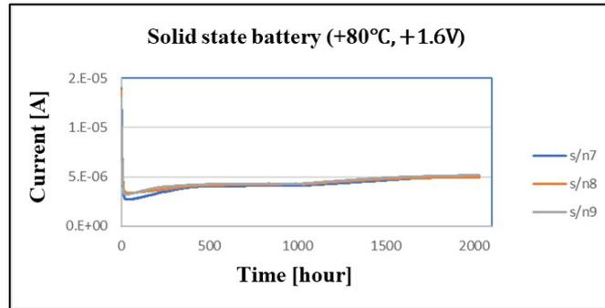
Fig. 36. The result of the ion migration test on solid-state battery
