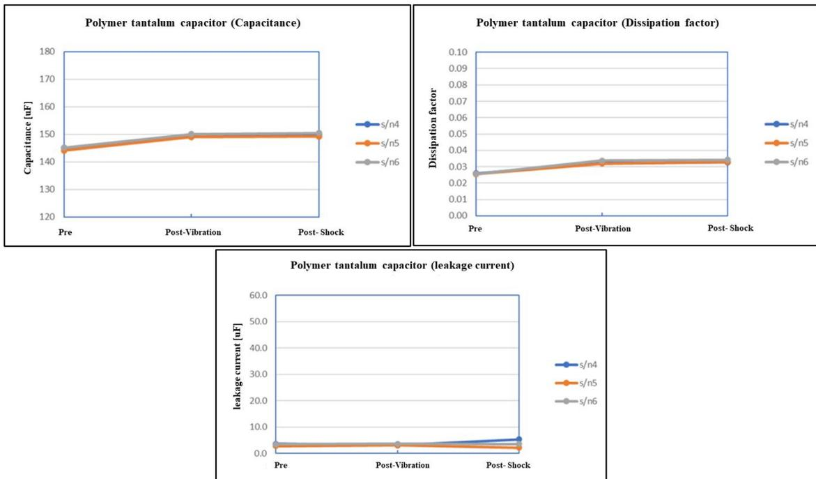
Fig. 10. The results of the electrical characteristic measurements after the vibration test and shock test on the polymer tantalum capacitor
