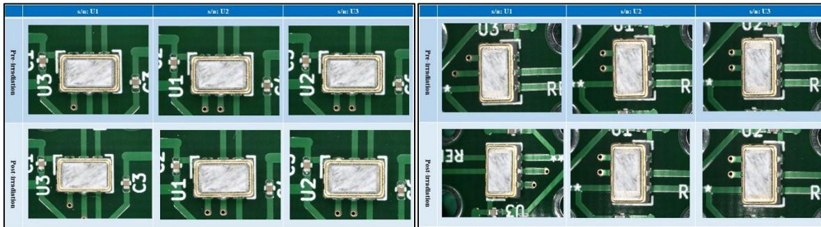
Fig. 7. The result of external visual examination after the TID test on the voltage-controlled crystal oscillator
