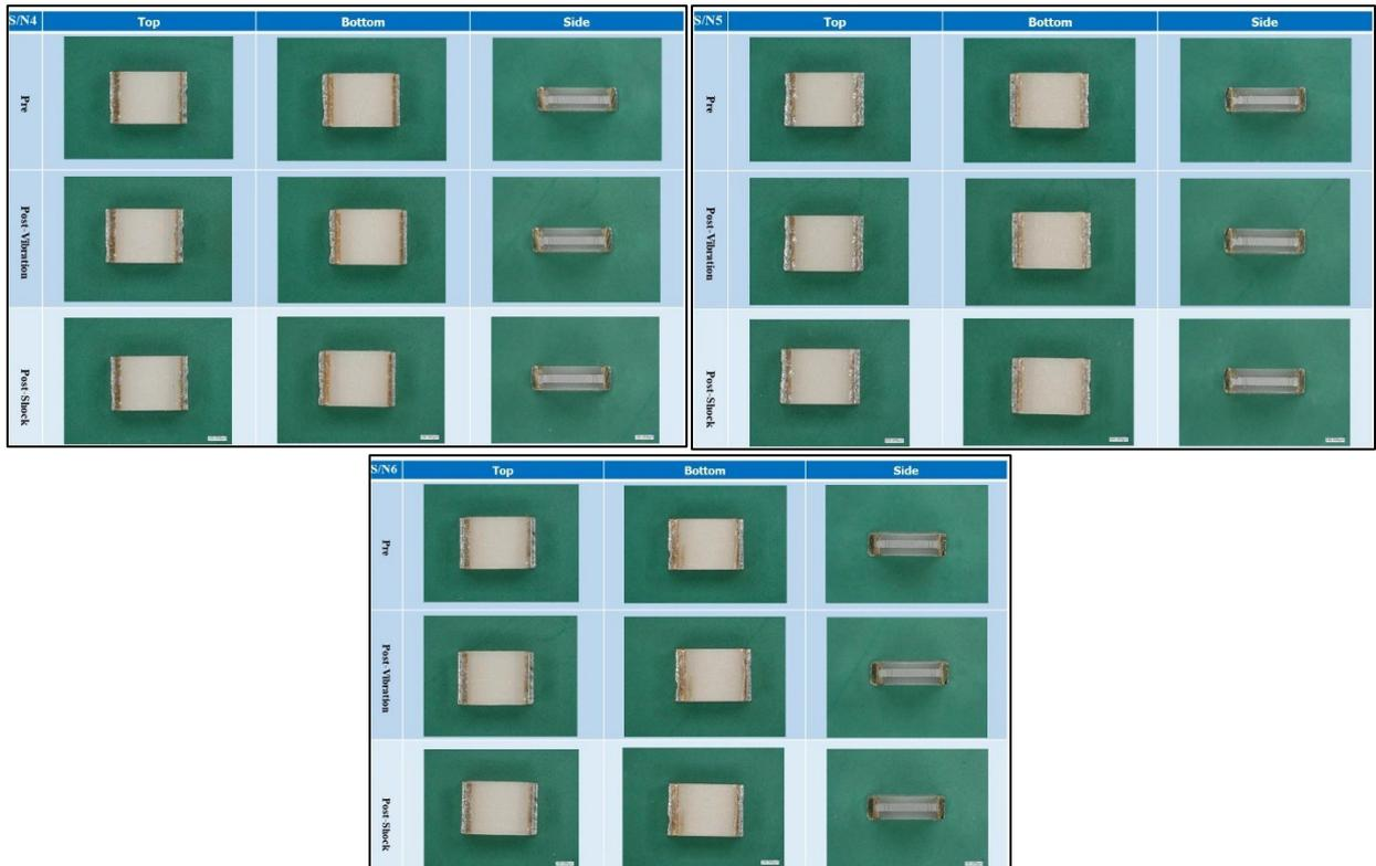
Fig. 13. The results of the external visual examination after the vibration test and shock test on the stacked metallized film chip capacitor
