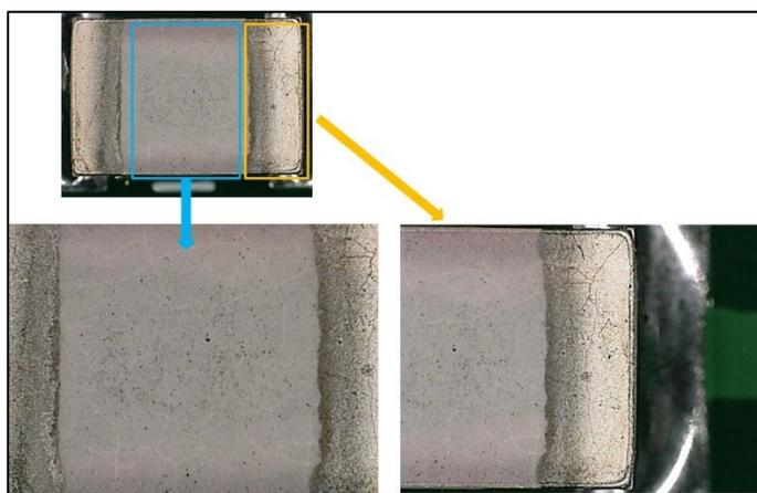
Fig. 18. Enlarged image of the solid-state battery sample(S/N:6) after shock test
