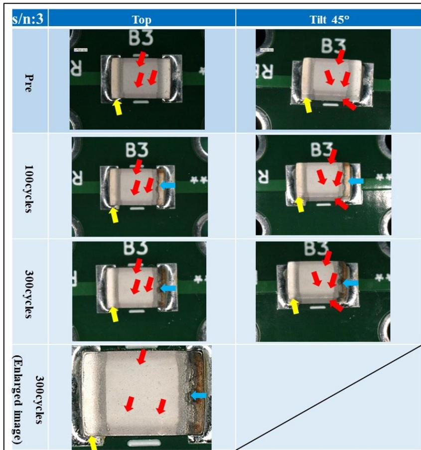
Fig. 35. The result of external visual examination after the thermal shock test on solid-state battery
