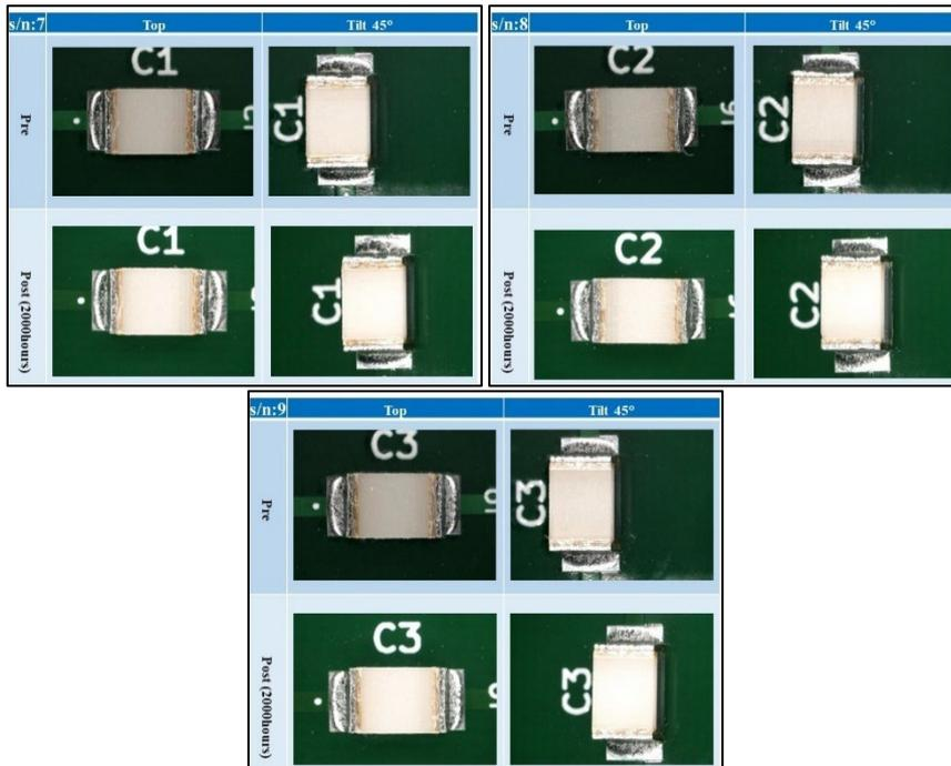
Fig. 28. The results of the external visual examination after the ion migration test on stacked metallized film chip capacitor
