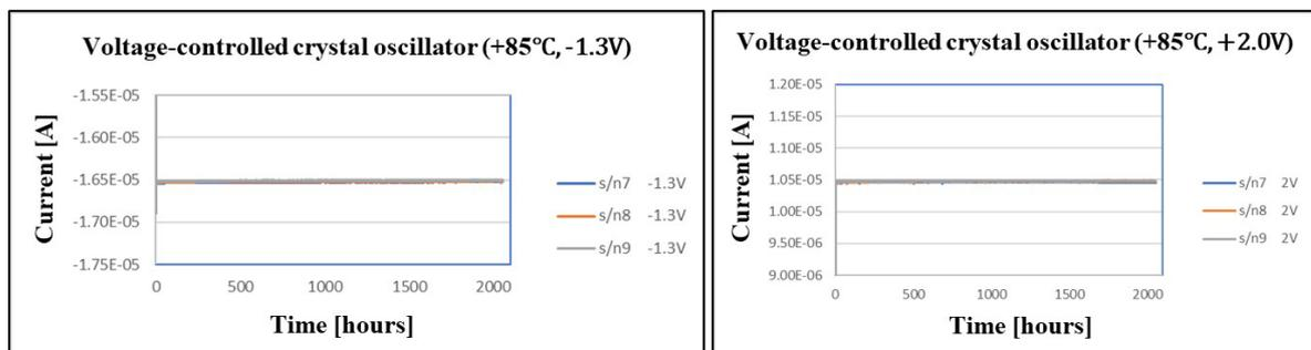
Fig. 31. The results of the ion migration test on the voltage-controlled crystal oscillator
