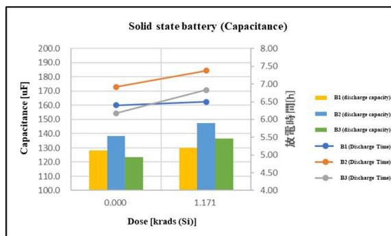
Fig. 8. The result of the electrical characteristic measurements after the TID test on the solid-state battery
