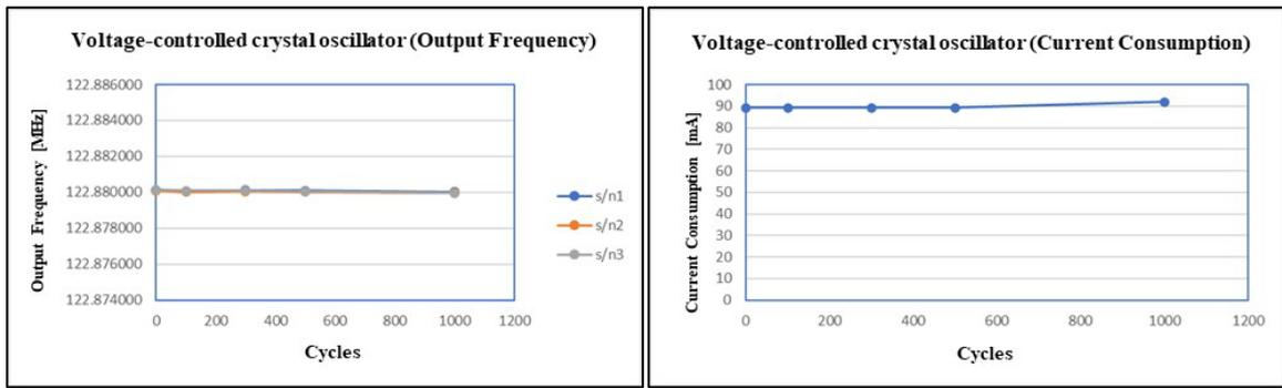
Fig. 29. The results of the electrical characteristic measurements after the thermal shock test on the voltage-controlled crystal oscillator
