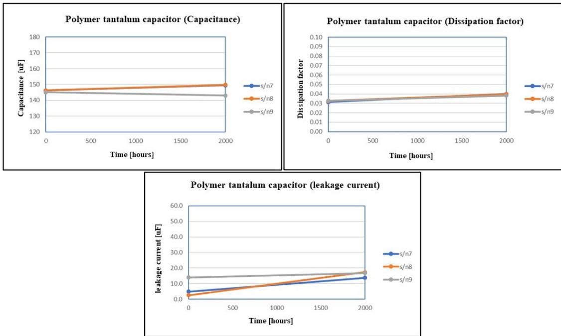
Fig. 22. The results of the electrical characteristic measurements after the ion migration test on polymer tantalum capacitor
