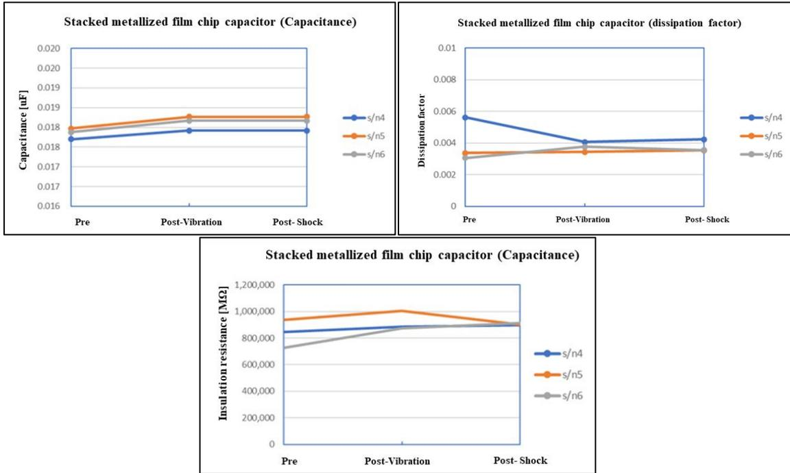
Fig. 12. The results of the electrical characteristic measurements after the vibration test and Shock test on the stacked metallized film chip capacitor
